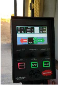
Figure 40. Muncie Advantage Plus Spreader Controller (Caltrans)
