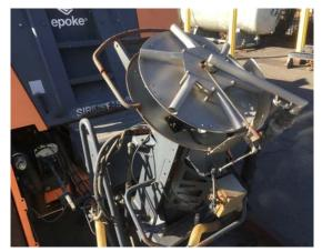
Figure 27. Epoke Brine Spray Spinner Applicator (Caltrans)
