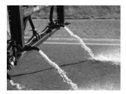
Figure 15. Direct Application Flood Nozzles (North Dakota DOT)
