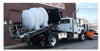
Figure 9. Snow Plow with Roll-Off Body Mounted Anti-Ice Spray System (Cliffside Body Corp.)
