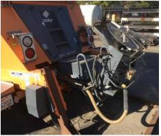
Figure 41. Kingvale Epoke Spreader Truck (Caltrans)
