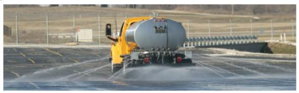
Figure 18. Multi-Lane Brine Spraying
