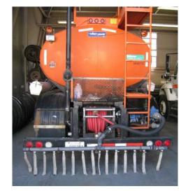
Figure 16. Kingvale Tanker Truck with Liquid Drip Tubes (Caltrans)
