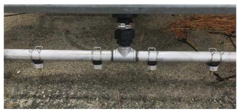
Figure 13. Simple Spray Bank with Clip-On Nozzles (Caltrans / VariTech)
