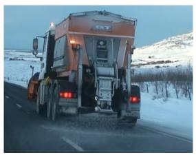
Figure 28. Epoke Pre-Wet Application (Epoke)
