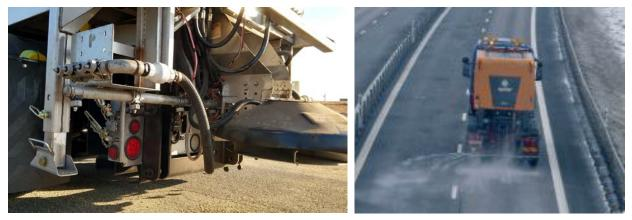
Figure 21. Henderson FRS Spray Attachment (Caltrans) Figure 22. Epoke Spray Bar Attachment (Epoke)
