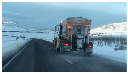
Figure 4. Sanding with Pre-Wet Treatment (Epoke)
