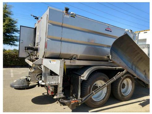
Figure 43. Caltrans Henderson FRS Truck Mounted
