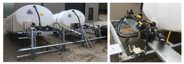
Figure 20. VariTech Industries Liquid Application Slip-In Systems (Caltrans, South Lake Tahoe)
