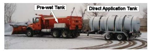
Figure 8. Truck Pre-Wet Spreader and Direct Brine Application Trailer (North Dakota DOT)
