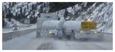
Figure 5. TowPlow Brine Highway De-Icing Operation (Caltrans)
