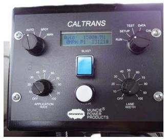
Figure 39. Caltrans Standard Muncie Spreader Controller (Caltrans)
