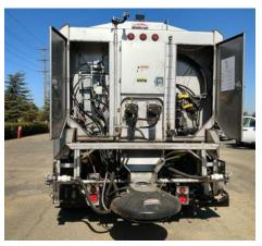
Figure 31. Henderson FRS Direct-Cast™ Pre-Wet (Caltrans)
