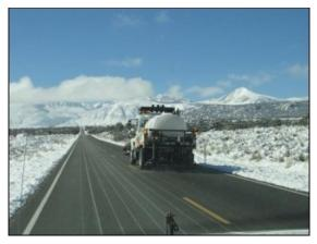
Figure 2. Highway Anti-Ice Treatment (Caltrans)
