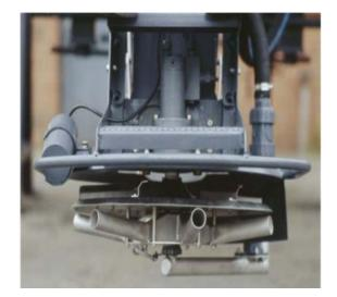
Figure 17. Liquid Spinner (Epoke)
