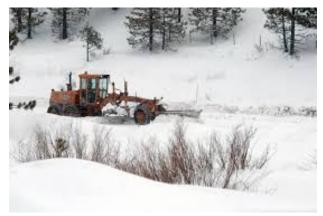
Figure 32. Caltrans Motor Grader Removing Bonded Ice Layer (Caltrans)
