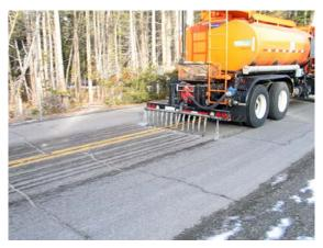
Figure 3. Brine Tanker Anti-Icing (Caltrans)
