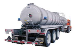
Figure 11. 2,700-Gallon Trailer-Mounted Anti-Ice System (Illinois DOT)
