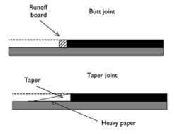
Figure 6.11 Transverse joints.
