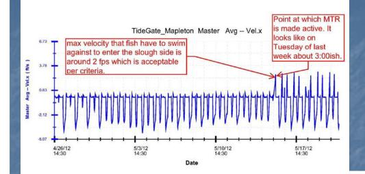
These graphs are a great data collection of a side-hinge gate operating w/out a regulator then the same gate operating with a regulator. As the data is a direct comparison (same gate, same waterway) it is very telling.
