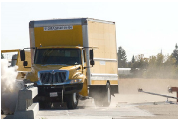
Image 5: Type 85 Bridge Rail: Van Body Impact
