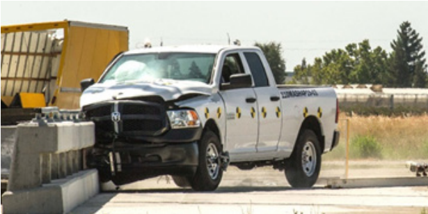
Image 4: Type 85 Bridge Rail: Pickup Truck Impact
