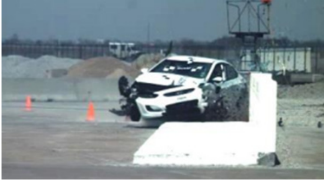
Image 3: MASH 1100C Small Car Test 3-20
