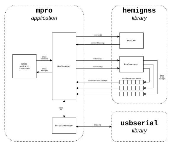
Figure 4.2: Simplified MPRO GNSS data flow
