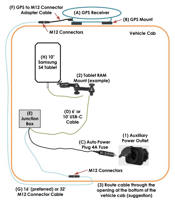
Figure 3.1: MPRO system wiring diagram
