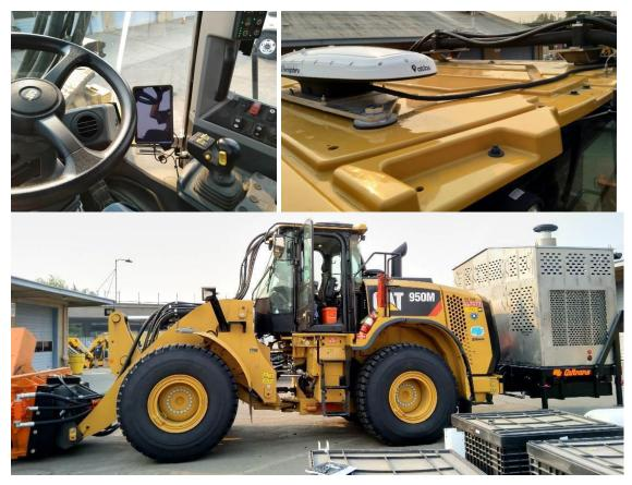
Figure 3.11: Caltrans Equipment #41870 2016 Caterpillar 950 front-end loader MPRO system installation
