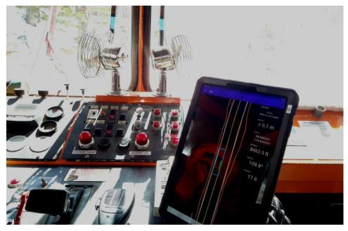
Figure 3.12: MPRO system with active HMI inside the snow blower. The operator's face was intentionally blurred out.
