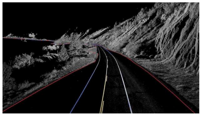
Figure 2.2: Example 3D laser scan point cloud with extracted base map overlay
