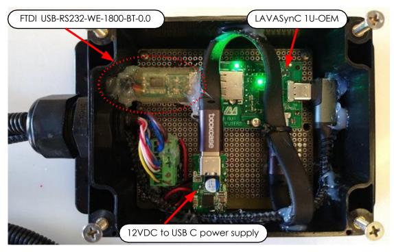
Figure 3.6: MPRO system power and data junction box inside view
