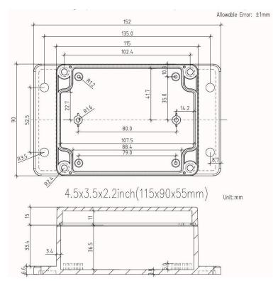
Figure 3.7: Part E Power/data junction box size and dimensions (not to scale)
