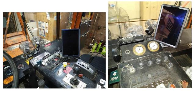
Figure 3.9: Example MPRO system installation inside a snow blower cab
