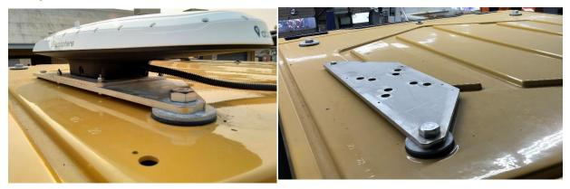
Figure 3.3: Vector V500 GNSS Smart Antenna custom-mounted on a Caterpillar 950 front-end loader with fiber glass roof
