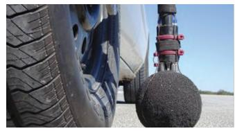
IMAGE 1: Measuring tire pavement noise
