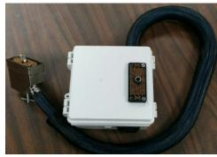
Figure 1: C1 Reader/Analyzer in Environmental Enclosure (closed)
