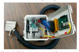
Figure 2: C1 Reader/Analyzer in Environmental Enclosure (open)d
