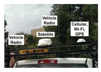
Image 2: Responder System Installed on Caltrans Vehicle
