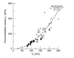
IMAGE 2: Relationship between preconsolidation stress and shear-wave velocity for clay.
