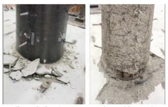
Figure 3: Cap beam concrete crushing and column flexural cracks (CFRP jacket removed) after hybrid simulation tests
