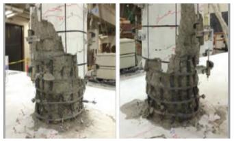
Figure 2: Column damage after cyclic tests
