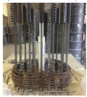
Figure 2: Column R-Calt-1 with couplers and new replacement longitudinal bar segments in place
