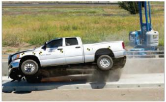
IMAGE 2: Pickup test impact
