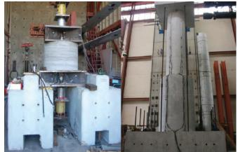
Figure 1: Bond-slip test Figure 2: Column-shaft assembly instrumented
