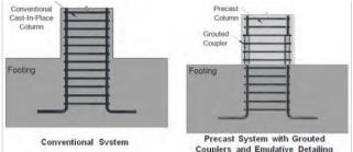
Figure 1: Comparison between conventional and precast systems with grouted coupler connections
