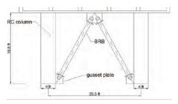
Figure 2: Transverse bridge bent with inverted-V
