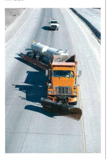
A TowPlow system in its deployed configuration
