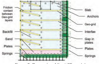
Figure 2: Geometry of the MSE model
