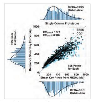
Figure 2: Comparison of the estimated shear key forces from the proposed method with reference forces from analyses (left, single-column bridges; right, two-column bridges)
