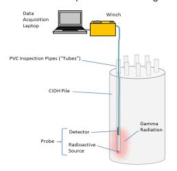
FIGURE 5: Gamma-Gamma Logging
