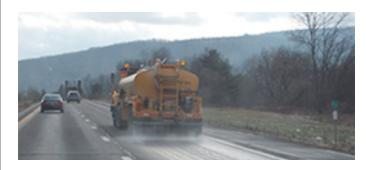
Image 2: Brine tank truck spreading salt brine on roadway
