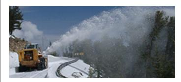
Image 1: Rotary blower removing snow from roadway
