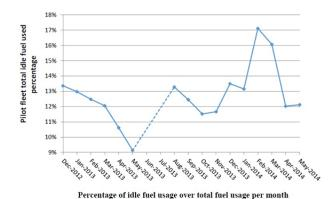
Image 8: Percentage of idle fuel usage over total fuel usage per month
