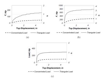
Figure 1: Comparison between capacity obtained with different load distribution: (a) medium-dense sand; (b) medium stiff clay; (c) granular cohesive soil
