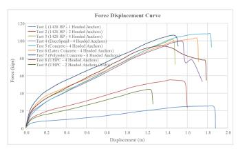
Image 5: Test results of shear force displacement response for all specimens
