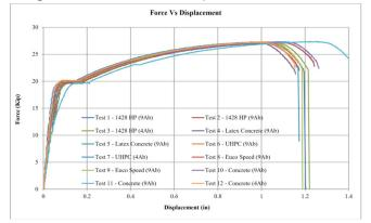
Image 7: Test results of pullout axial force displacement response for all specimens
