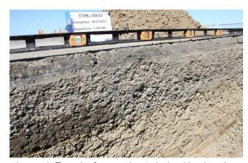
Image 1: Test pit after accelerated wheel load testing on FDR section with foamed asphalt and cement stabilization. An equivalent of 34 million ESALs was applied to this section, resulting in 6mm of rut, but no cracking
