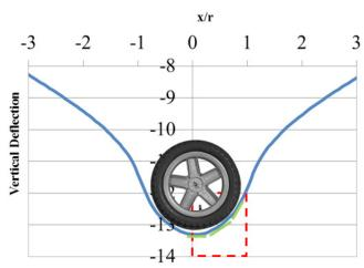
Image 1: Exaggerated pavement deflection model
