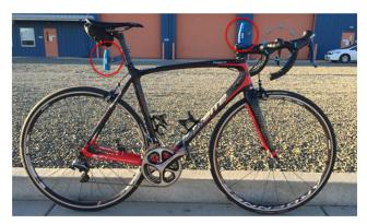
Image 1: Road bicycle instrumented with accelerometers (solid red circles) and a Global Positioning System (GPS) unit on the handlebar (circle of blue dashes) used to obtain bicycle vibration measurements.
