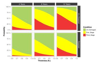
Image 1: Slab performance sensitivity with thickness changes
