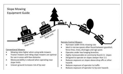
Figure 1: Guide showing slopes and conditions relevant to mower equipment selection
