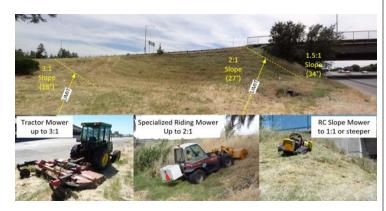
Figure 2: Mowers on typical roadside slopes
