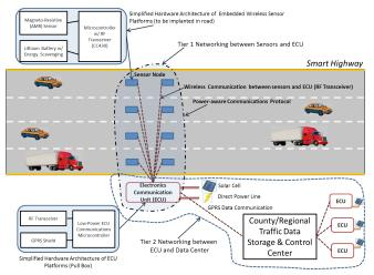
FIGURE 1:Proposed Architecture for Smart Road Sensing Networks
