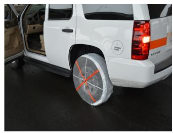
SUV with the cloth tire traction control device installed on the rear wheels
