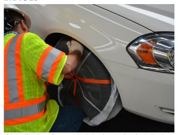
Cloth tire traction control device being installed on the car
