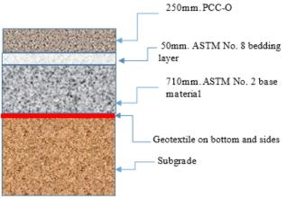
Figure 2: Concrete Test Section Design
