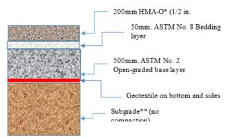
FIgure 3: Asphalt Test Section Design
