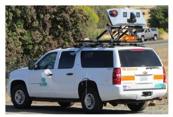
FIGURE 1: MX8 mobile terrestrial laser scanner system mounted on a Caltrans vehicle
