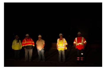
Image 1: 25 Feet from Light Plant Only Car Lights (left to right) Old PPE Rain Jacket ; New PPE Rain Jacket; Non-retroreflective Maintenance Clothing; Old PPE Vest; and New PPE Vest and Pants combo.
