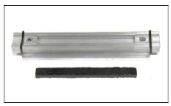
Image 3: Modified mold configuration and beam specimen
