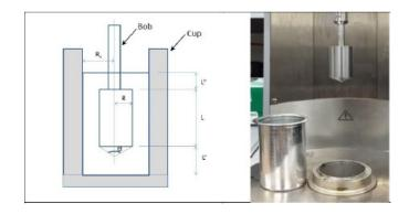
Image 1: Concentric cylinder geometry
