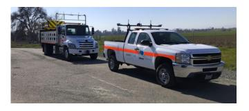
Image 4: The Caltrans ATMA performance testing system
