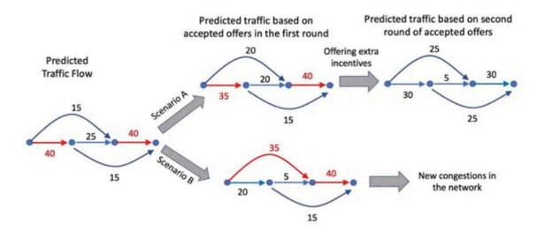
Figure 2: Two different incentive offering strategies with two different outcomes. Scenario B leads to the creation of new congestions in the network. The number on each edge shows the number of cars on that particular road/edge. The red edges show the congested roads.
