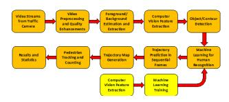
Image 1: End-to-end system architecture
