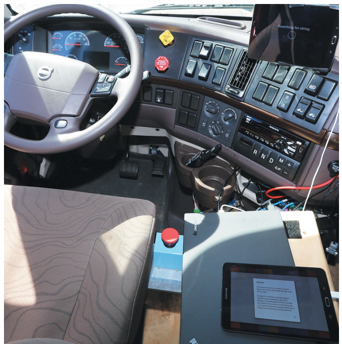
In the cab of a truck equipped with Cooperative Adaptive Cruise Control technology, drivers monitor an interface tablet screen at left. A shut-off device, with red button, is positioned at center.
