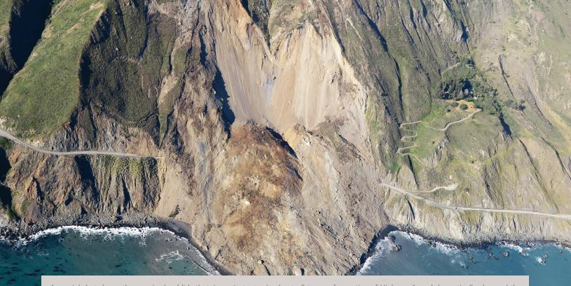
An aerial shot shows the massive landslide that, in an instant, wiped out all traces of a section of Highway 1, and dramatically changed the surrounding landscape along the Big Sur coast. Recognizing the highway's importance, Caltrans almost immediately began plans for rebuilding.
