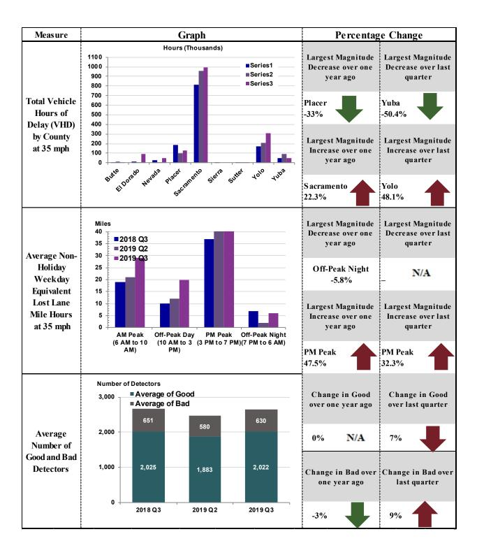
Note: As is identified by the detector health graph above, the District's detector health has declined. The graphs indicate a 7% reduction in the number of Good detectors. Caltrans has a Traffic Monitoring Station project (EA: 3F840) completed to help improve detector health. Two other projects will cover locations that were missed by this and other previous projects. We had informed our electrical unit of the declining number of detectors and that they will need to be replace/reactivate.
