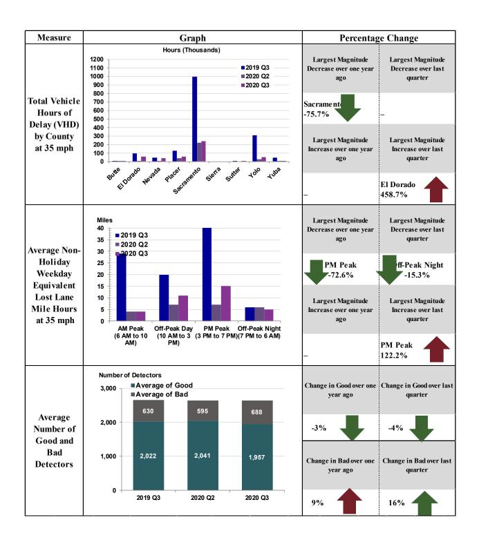
Note: As is identified by the detector health graph above, the District's detector health has worsened. The graphs indicate a 4% decrease in the number of Good detectors, comparing with previous quarter. Caltrans has a Traffic Monitoring Station project (EA: 3F840) completed to help improve detector health. Two other projects will cover locations that were missed by this and other previous projects.
