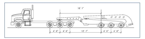
Figure A. The tractor and the jeep are not close coupled. The two closest tractor drive axles are at least 18'1" from the closest jeep axle. The same is true for rear tractor axle and two closest jeep axles.
