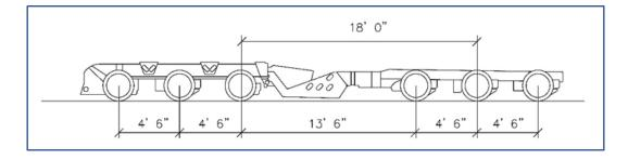
Figure B. The trailer and the Mechanical Distribution Unit (MDU) are close coupled. The closest trailer axle is not at least 18'1" from the two closest MDU axles. The same is true for the two rear trailer axles and the closest MDU axle.
